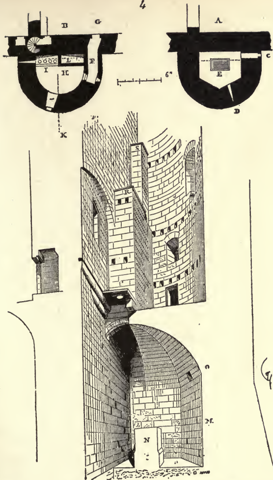
Fig. 381. Latrines in the Castle of Pierrefonds, France.*
